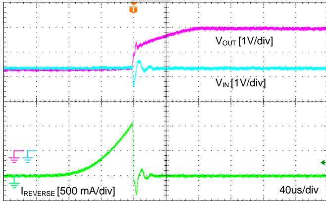
**Figure 22. Reverse Current Blocking at Switch On**
