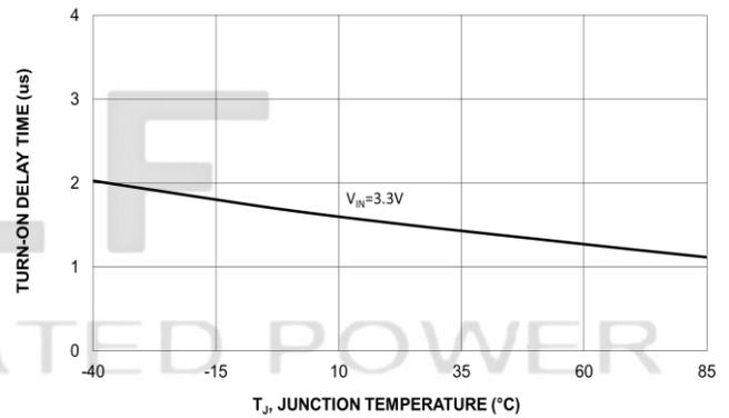
Figure 17. Turn-On Delay Time vs. Temperature, GLF72122
