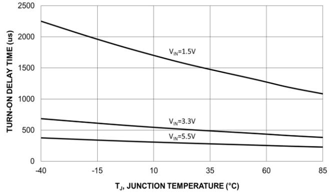
Figure 15. Turn-On Delay Time vs. Temperature, GLF72120
