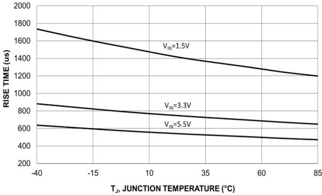
Figure 14. V<sub>OUT</sub> Rise Time vs. Temperature, GLF72120
