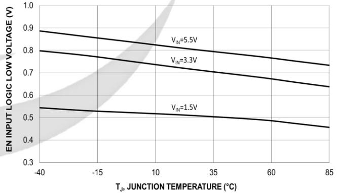
Figure 13. EN Input Logic Low Threshold Vs. Temperature
