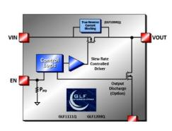
Santa Clara, CA — October 6, 2022 — <u>GLF Integrated</u> <u>Power</u>, manufacturer of innovative ultra-low-power load switches, is pleased to introduce two new Automotive grade AEC-Q100 I<sub>Q</sub>Smart<sup>™</sup> load switch ICs. The AEC-Q100 qualified <u>GLF1111Q</u> and <u>GLF1200Q</u> are rated for a wide temperature range (Grade 1 -40°C to +125°C). The
